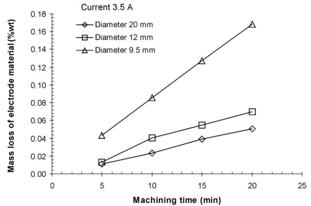
Fig. 4. Percentage of mass loss of electrode material at a current setting of 3.3 A.
